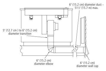
THROUGH FLOOR BETWEEN JOISTS TO OUTSIDE
